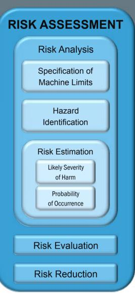
In order to analyze risk, three elements must be combined and considered; the specification of the limits of the machine, identification of hazards, and risk estimation. Together, these attributes are considered to define a level of risk, which is then evaluated to determine whether the risk reduction objectives have been achieved, also known as achieving tolerable (or acceptable) risk.
